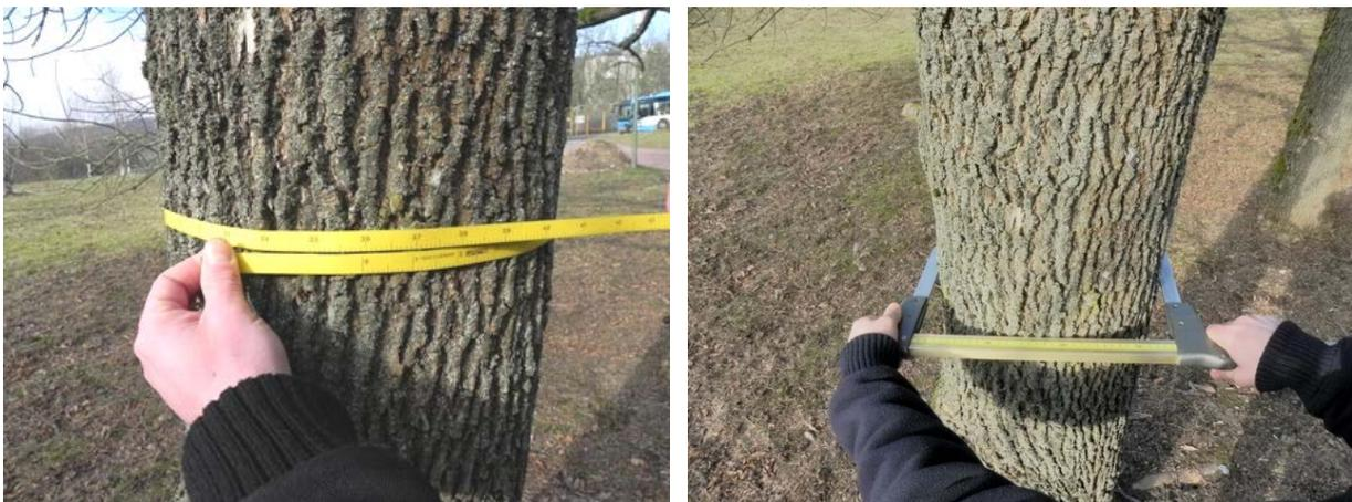
Measuring DBH with a diameter tape (left) and a diameter calliper (right).
