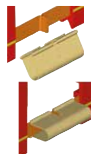
Mounting the connector Cu-C
