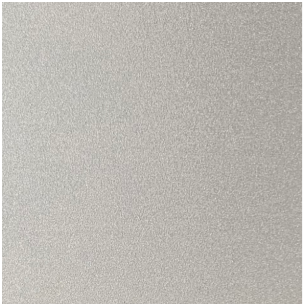
MAT.01 FACADE CLADDING ALUCOBOND JLR CHAMPAGNE METALLIC ALUMINIUM SHEET https://www.alucobondusa.com
